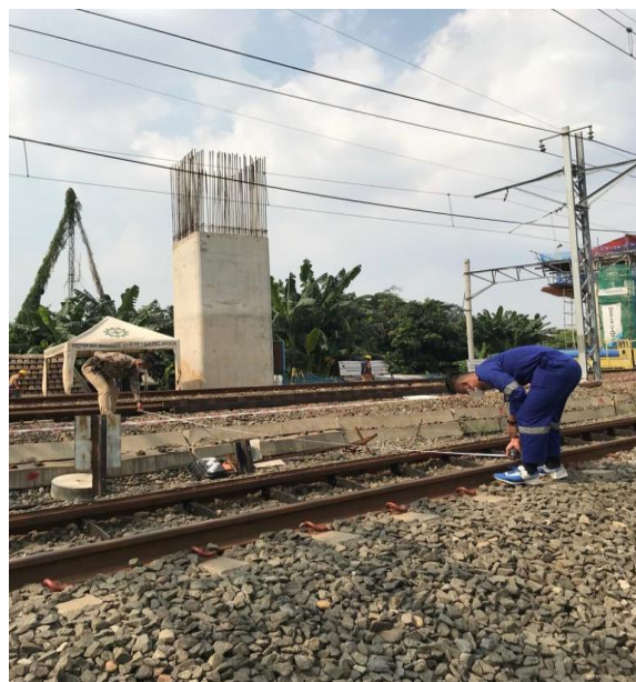
Gambar V. 16 Pengukuran pergeseran track
