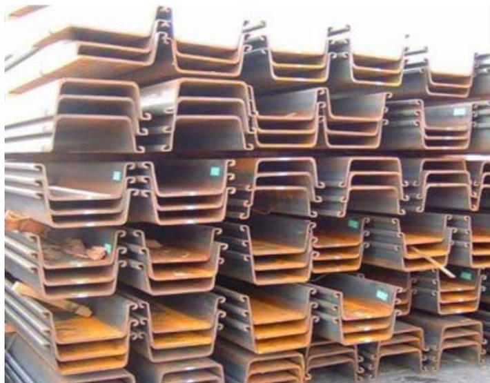
**Gambar III. 6** *Sheet Pile* Baja
