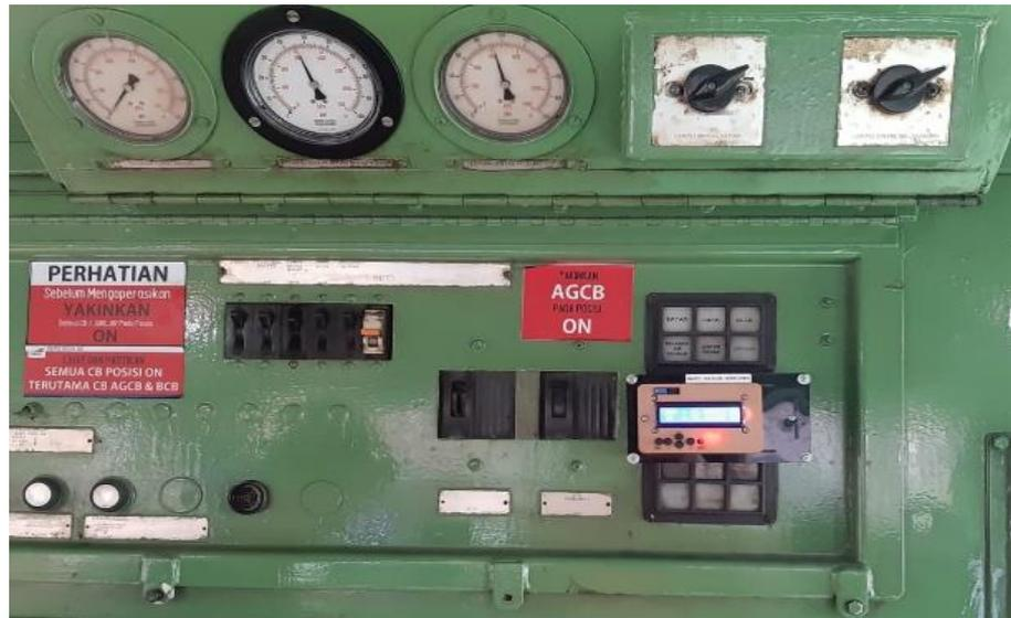
**Gambar V. 4** Alat Smart Voltage Monitoring Dalam Kabin Masinis
