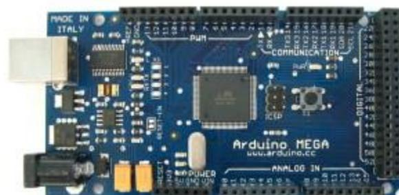
**Gambar III. 4** Arduino MEGA
