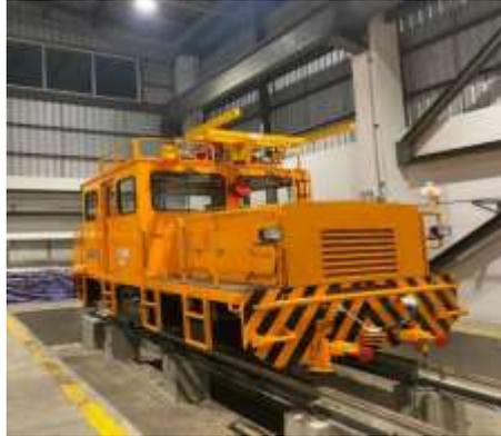
**Gambar II.5** *Motor Car With Crane*
