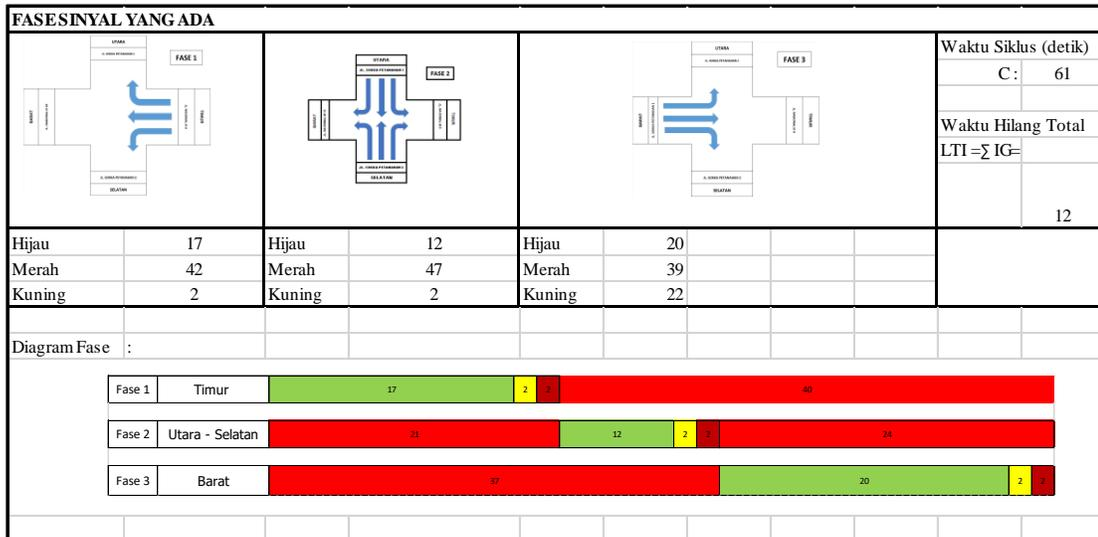
**Gambar V. 21** Diagram Fase Simping Sokka Baru Usulan II (3 Fase)
