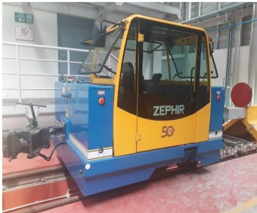
**Gambar II. 7** *Shunting Locomotive*
